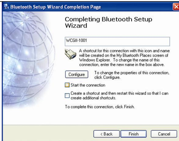
5. In the Bluetooth Setup Wizard Completion Page, uncheck the box for Start the connection. Then click on Configure.
