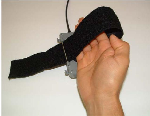
Secure the arm band by pulling on the end as shown. Fold the strap back around and secure via the Velcro strips at the end of the strap.
