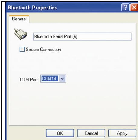
4. In the Bluetooth Properties window, uncheck the box for Secure Connection and then click OK.
