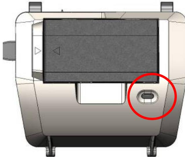
When power is off, slide the battery locking slider to the left-most position. Grab the battery on both sides. Tilt the battery, then pull it straight out. The latching mechanism prevents battery removal unless it is tilted first.
