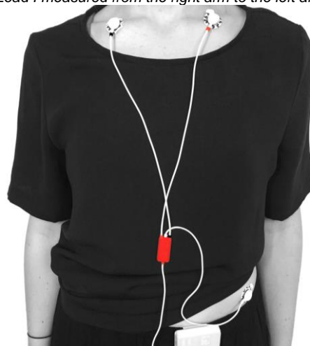
Fig. 4. Example of an assembled ECG placement with IN+ & IN- on the collarbones acc. to Einthoven Lead I from right arm to left arm and REF on the iliac crest.
