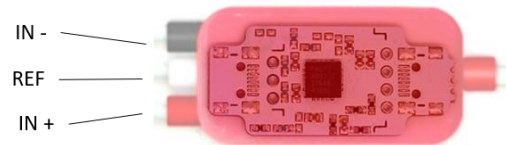
Fig. 2. Assembled ECG sensor – from the inside.
