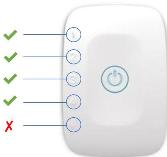
Figure 6: ECG compatible biosignalsplux channels (green checkmarks).
