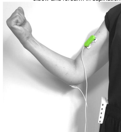
Fig. 4. Example electrode placement of the assembled version along the muscle fibers.
