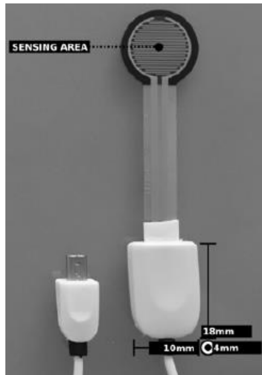
Fig. 1: Type 3 FSR sensor with a arrange up to 10 Kg
