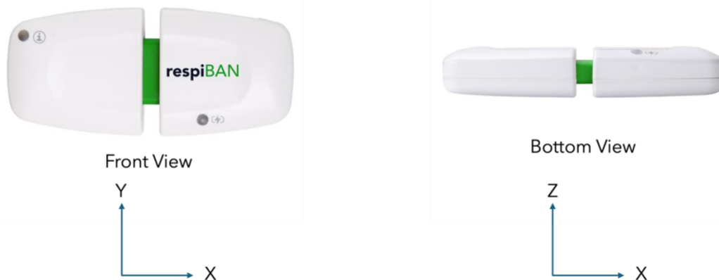
Figure 3: respiBAN motion sensor axes.
