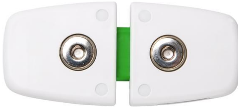
Figure 2: Backside of the respiBAN wearable with the two stud connectors.
