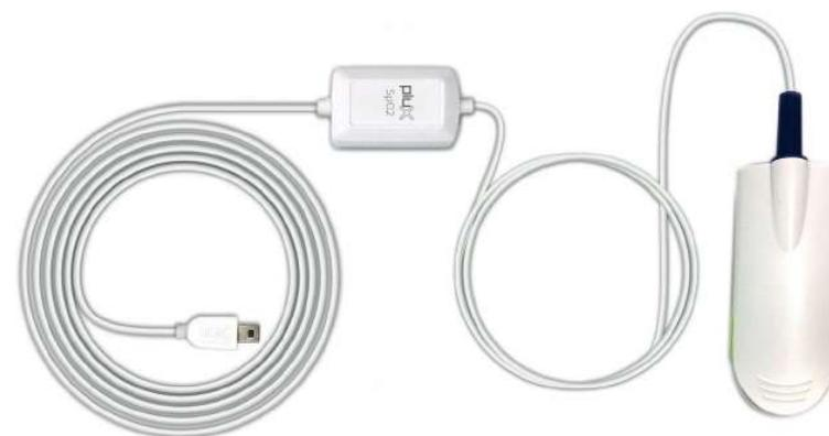
*This sensor can be used to estimate the blood oxygen saturation level in the finger with +/- 2% accuracy compared to a medical sensor.*
