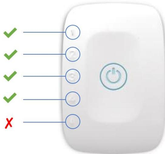
Figure 5: LUX compatible biosignalsplux channels (green checkmarks).
