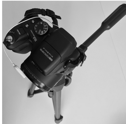
Fig. 2. LED used on a camera lens for synchronization.
