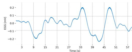
Fig. 2 Typical unfiltered EGG output (with subject at rest and presenting basal gastric activity)
