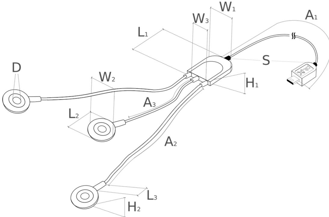
Fig. 4 Physical characteristics of the standard EGG sensor.
