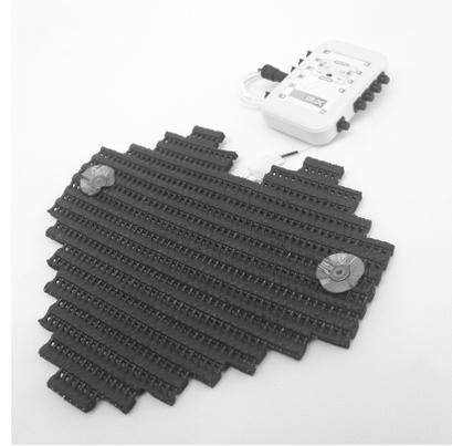
**Fig. 3.** Experimental apparatus consisting of the sensor pad with a heart shaped form factor, where a pair of Ag/AgCl electrodes are integrated, and a biosignal acquisition device.
